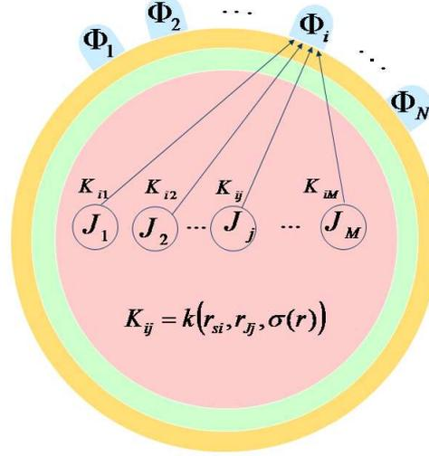
**Figure 2.4:** Geometric representation of the forward problem. A three-shell spherical head model,  $M$  current sources and  $N$  voltage measurements
