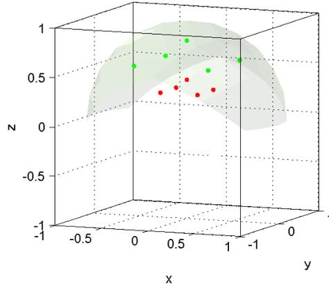
**Figure 4.2:** Grid points of the solution space consisting of 2 spherical layers of 5 electrodes each.
