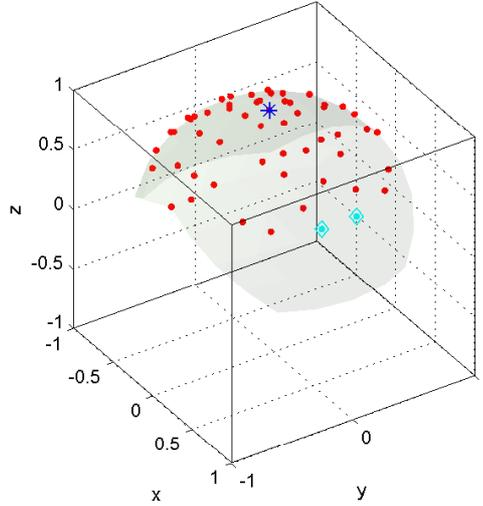
**Figure 4.1:** Graphical representation of the electrodes position used to compute the measurements for the evaluation of the methods. Electrode marked with "\*" represents  $Cz$  and electrodes plotted as "◇" represent  $Fp1$  and  $Fp2$
