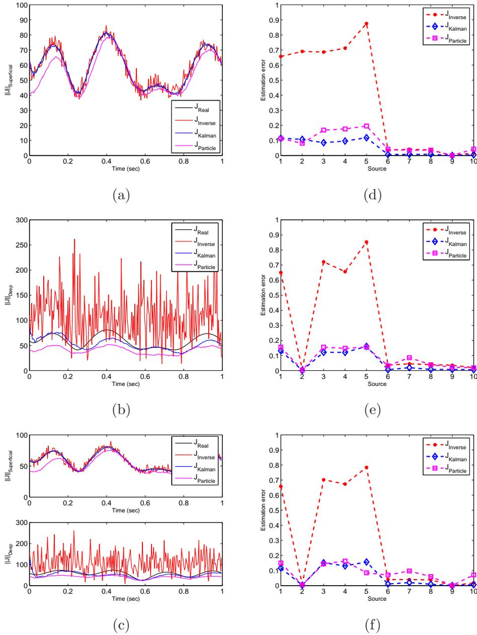
**Figure 4.3:** Left column: Magnitude of the real and estimated sources, (a) single active superficial source, (b) single active deep source and (c) two uncorrelated active sources. Right column: Estimation error for the whole source space given by the three methods, (d) single superficial active source, (e) single deep active source and (f) two uncorrelated active sources.
